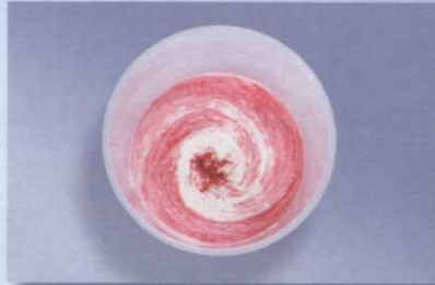
Clay and pigment mixed at 30% self-rotation.
