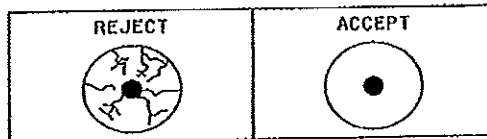
FIGURE 2009-3. Cracked glass surface.
